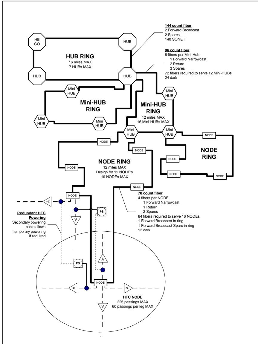
*(Note the Redundant HFC Powering showing one power supply supporting two nodes)*
